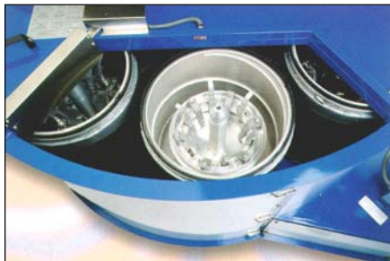
For loading and unloading the hydro-heads of the Hydroc stand still
