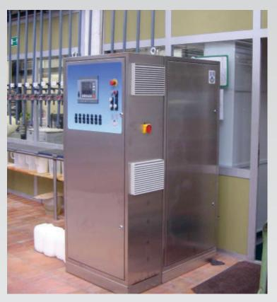
Each module can be placed independently somewhere inside the factory so that also complicated layouts can be realized. For example, one chemical dispensing module can supply two dyehouses by using two distribution modules.
