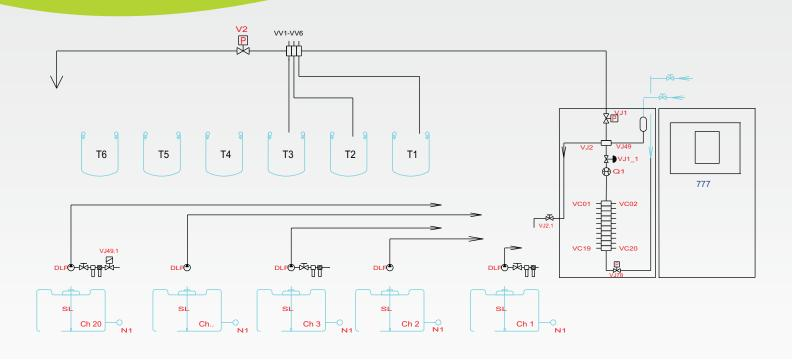
The heart of the Chemical Dispensing Module is the Coriolis flowmeter, which measures the mass going through the flowmeter accurately (up to 0.5 % of the requested amount, depending on the amount being measured).
