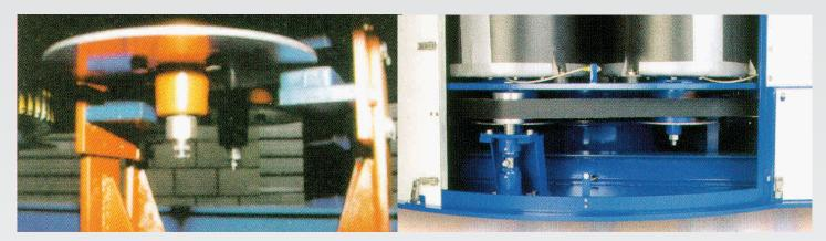
This type of brake has the advantage that no indefinable forces affect the pulleys, rubber bearings and ball bearings. Due to the contact-free braking the noise level is reduced remarkably. The brake does not need maintenance. The loading height of one meter above floor level is optimal for ergonomic loading and unloading. The hydro-extractor and RF dryer can be operated by the same person.
